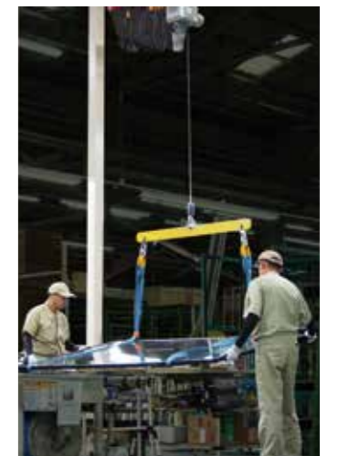
Invert large window glass by using only one sling belt
