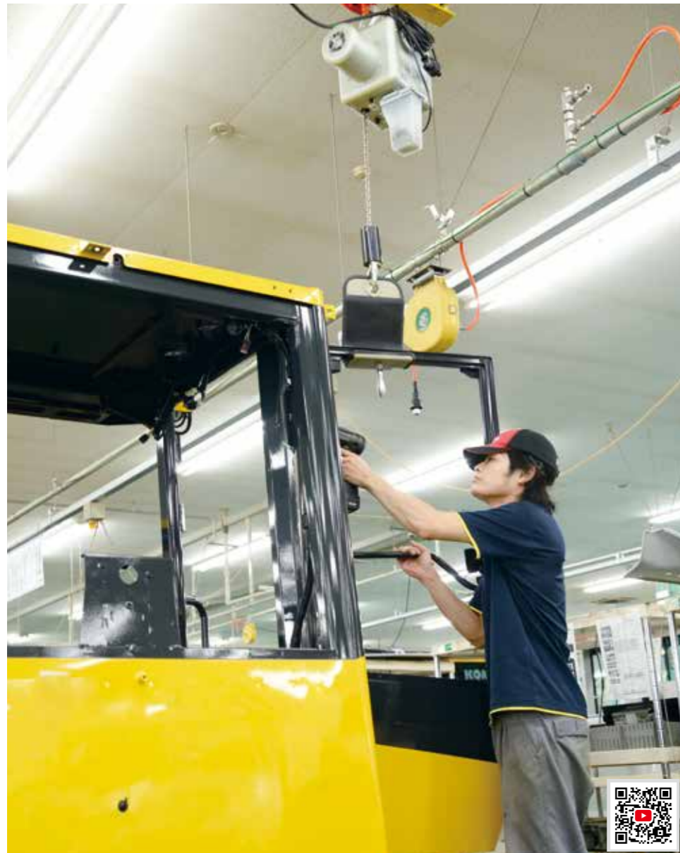
Bolt tightening work that used to be done by two persons can now be done by one
